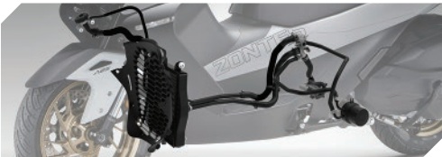
Water/Oil Dual Cooling System
