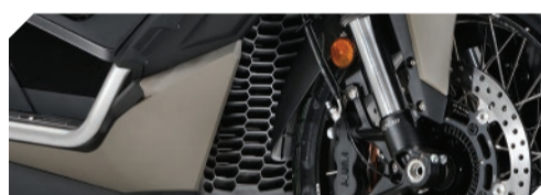
Water/Oil Dual Cooling System
